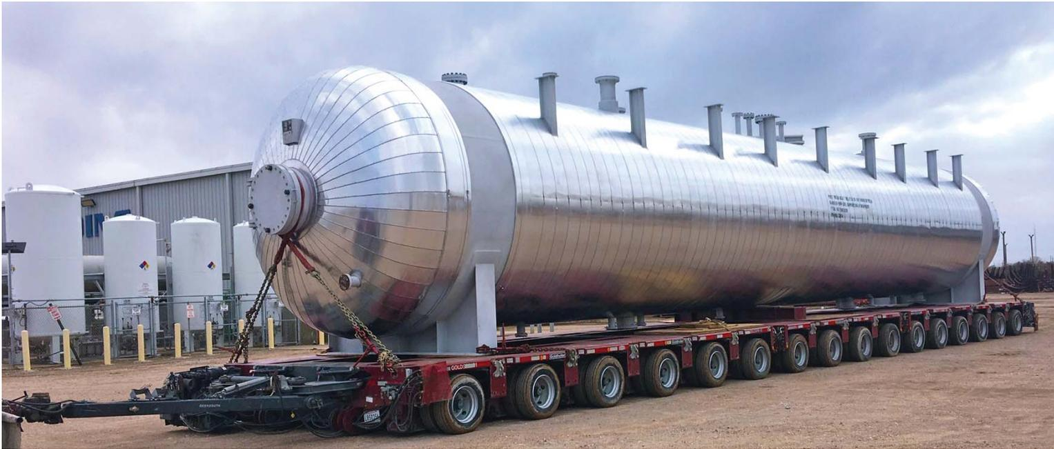
EDGE I (Enhanced Deep-Grid Electrical) is Forum's widely deployed desalting/dehydrating solution, sharing the same technical foundation as the EDGE II/EDGE III options. Every detail is meticulously crafted to create the industry's most effective solution for removing water and contaminants – sodium, calcium, magnesium chloride & others – from crude oil.
