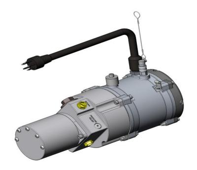
This small Hydraulic Power Unit (HPU) delivers 4 Lpm / 1 usgpm at adjustable pressures up to 200 bar / 3000 psi and is suitable for powering manipulators, tools etc.
