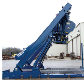
Conventional A-Frame 1217 5.6 tonnes luffing rating 7 tonnes overboard rating
