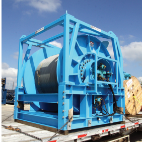
421 ROV Winch System 3,000 Meter Medium Duty ROV Winch
