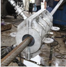
Tuff Coat M Marine Lubrication Systems Tuff Tool Lubricator installed on a wire rope
