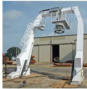
Conventional A-Frame 952 16 tonnes luffing rating 30 tonnes overboard rating
