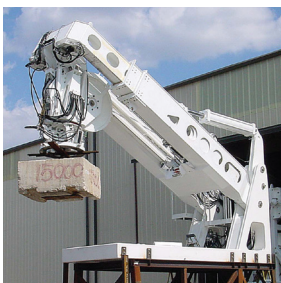
Telescoping Launch & Recovery System 1015 13.5 tonnes luffing rating 22 tonnes overboard rating
