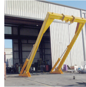
General Purpose A-Frame 474 4.5 tonnes luffing rating 7.5 tonnes overboard rating
