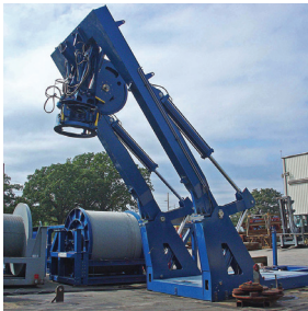
Self-Erecting A-Frame 966 13.5 tonnes luffing rating 22 tonnes overboard rating
