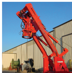
Telescoping Launch & Recovery System 7021 10 tonnes luffing rating 20 tonnes overboard rating
