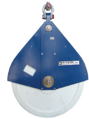
Overboard Sheave P19 1,500 kg safe working load 483 mm sheave tread diameter
