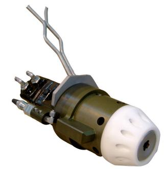
The sensor section directly measures the torque between the reaction lugs of the tool and the driven shaft. The sensor is a strain gauge bridge optimized for torsion measurement. When the tool is fitted with the paddle type socket, the torque reaction is taken through the manipulator handle but still measured by the sensor.
