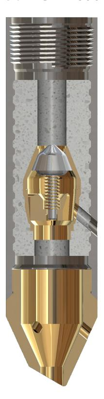
The Davis-Lynch™ 501ECN float shoe features PVTS check valves and an eccentric nose. Down-jet ports improve circulation, turbulence and even distribution of fluid for well cementing applications even in challenging conditions. Since Forum's purchase of Davis-Lynch over 3,000 501ECN float shoes have been run.
