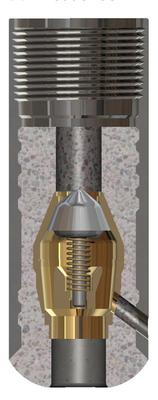
The Davis-Lynch™ 501 float shoe features PVTS check valves and standard cement noses and non-standard noses. Down-jet ports to improve circulation, turbulence and even distribution of fluid for well cementing applications even in challenging conditions. Since Forum's purchase of Davis-Lynch over 7,750 501 series float shoes have been run.
