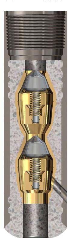
The Davis-Lynch<sup>TM</sup> 501DV float shoe features PVTS check valves and standard and non-standard cement noses. Down-jet ports improve circulation, turbulence and even distribution of fluid for well cementing applications even in challenging conditions. Since Forum's purchase of Davis-Lynch over 5,000 501DV float shoes have been run.
