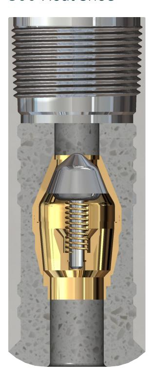
The Davis-Lynch™ 500 float shoe features PVTS check valves which will withstand 24 hours of circulating time with 12 ppg fluid at 10 bpm, and is rated to 5,000 psi back pressure at 400°F. Since Forum's purchase of Davis-Lynch over 21,000 500 series float shoes have been run.
