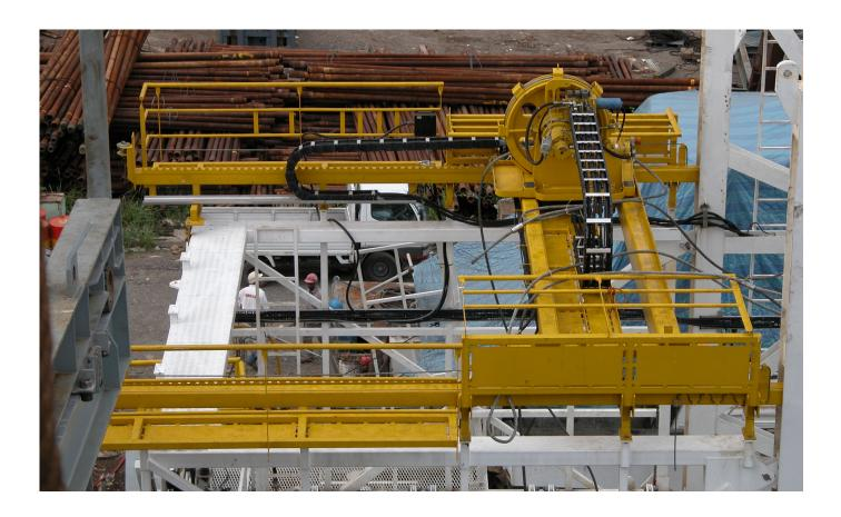
Forum Energy Technologies' offline activity crane (OAC) is a compact, fit-for-purpose derrick or mast-mounted hoist that facilitates a seamless standbuilding operation. The OAC hoists and racks drillpipe, tubing and casing, ranging from 2 7/8 to 13 5/8 in.
