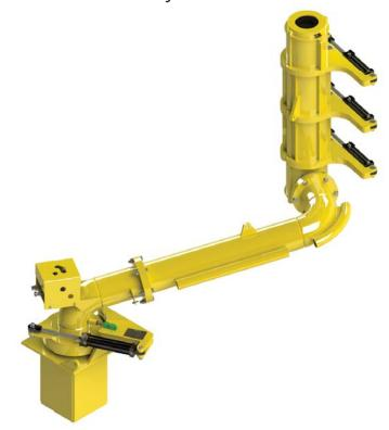
The P-Quip self supported mud bucket is hydraulically operated. It requires only one action to swing it in to position, close it, and lock it around the drill string. The operator simply pushes the control lever forward to close the bucket and pulls it back to open it. Letting go of the lever at any time will instantly stop the movement.
