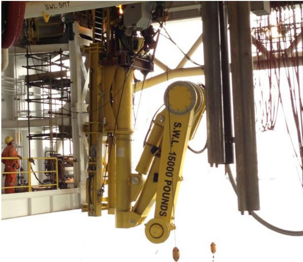
The Forum Energy Technologies multipurpose crane (MPC) is a highly versatile and valued addition to any rig. Hydraulically actuated, the MPC provides multi-axis control to access hard-to-reach places, virtually eliminating the need for manual interface.
