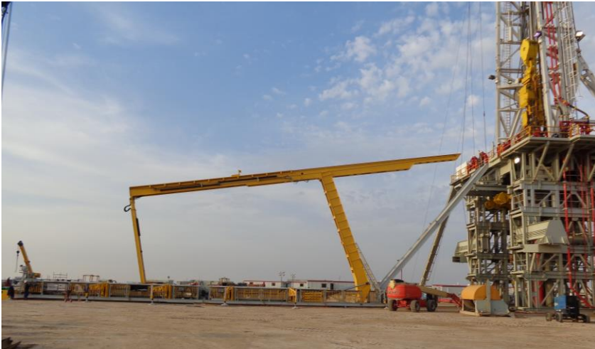
The Pipe Wranglers Model 5000 catwalk easily accommodates the taller rig floor of rigs in the Middle East.
