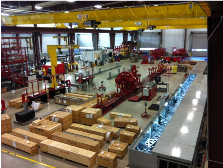
Forum's lean manufacturing facility (left: component assembly area; center: torque machine; right: hydrostatic test bay)
