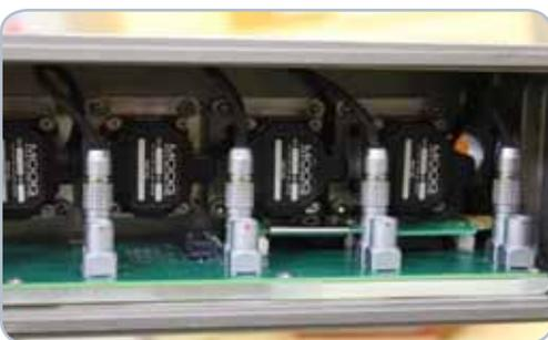
The in-arm electronics module features diagnostic lights that indicate system health.
