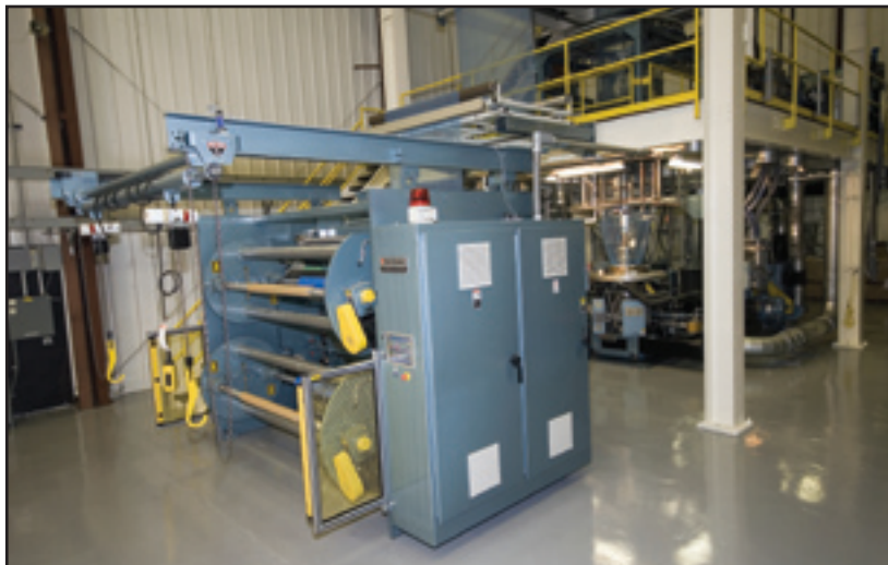
The blown film lab line in New Jersey is being used for trials to support markets in stretch hood, lamination films, shipping sacks, GP film and technical films.
